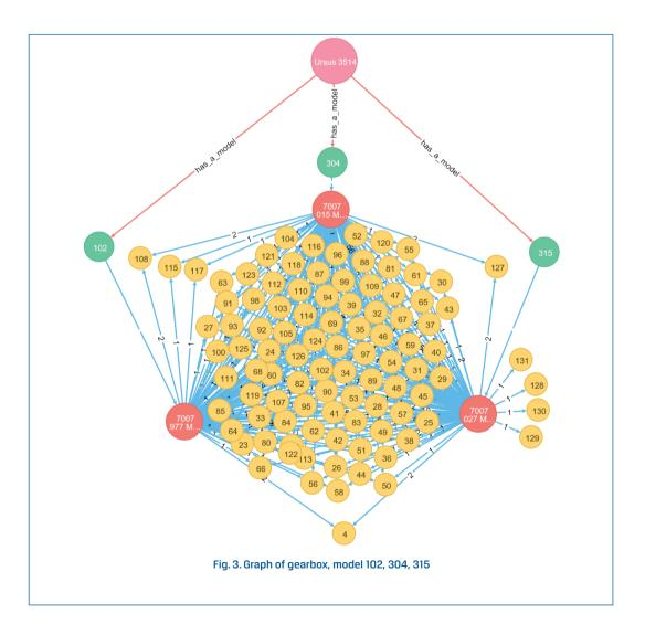
Graph in Fig. 3. is too big to display readable names of gearbox parts and components. When the graph is displayed on the screen in Neo4J, then after clicking on chosen node, thanks to graph reactiveness, all descriptions of each node like node name and other properties can be found out. Such possibility is shown in Fig. 4.,
