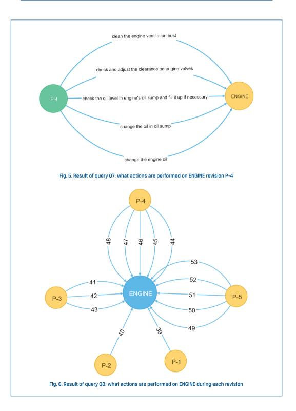
The relation in Fig. 6 represent actions of technical revisions operations listed in Table 1. For example: relation 49 means "check the oil level in engine's oil sump and fill it up if necessary". That information is available due to the graph interactive or a query.
